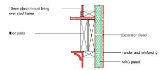
iii. Install 'Render Expansion Bead' between both Greenboard™ surfaces, applying a bead of No More Nails to both internal surfaces of bead. Press into position, scrape off excess glue, and tack fix until dry.
